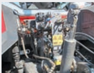
The spools have good caps and relief levers. Labelling also good.
